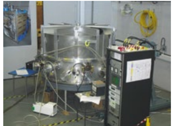
Figure 3 (right). The KMOS main cryostat undergoing its first cooldown cycles. The closed-cycle coolers are visible around the base of the cryostat; the remaining ports contain the feedthroughs for some of the 1500 electrical connections into the cryostat. The electronics rack to the right contains all the housekeeping electronics and will eventually be mounted on the Nasmyth platform.
