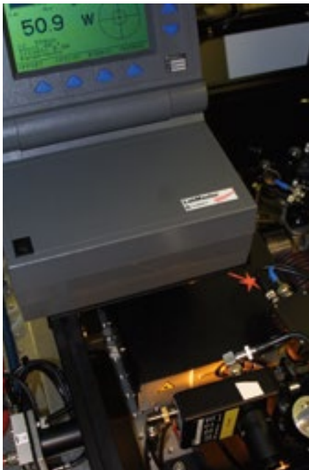
Figure 14. 50.9 W CW at 589 nm obtained from the three-way free-space CBC, as shown by the display.
