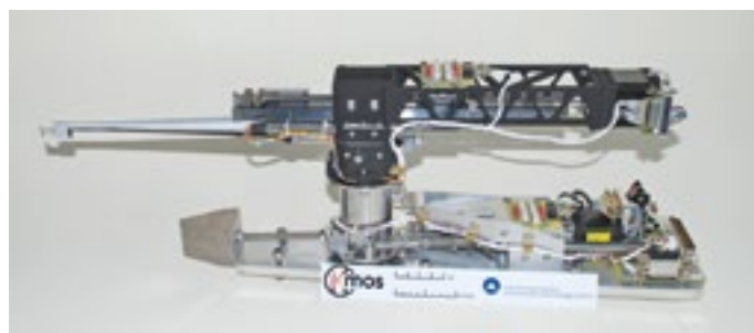
Figure 4. One of the fully assembled KMOS pickoff arms. The linear motion is a stepper motor drive in the top of the arm, and the angular motion is a stepper drive in the base. The total length of the mechanism is \sim 50 cm.
