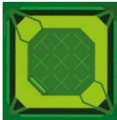
Figure 1. Picture of a single bolometer used in the actual version of SABOCA. The thermal conductivity depends on the thickness and number of “legs” connecting the central part of the membrane with the outside. Other layouts were produced and even tested but not used finally. All bolometers have cross-dipole absorbing elements.
