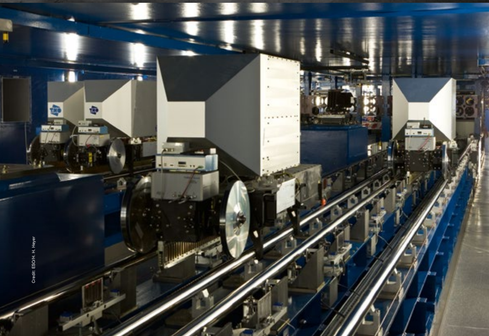
Two contrasting images of a section of the VLT interferometric tunnel. Upper: as it appeared ten years ago. Lower: as it appears today filled by four of the Delay Lines.
