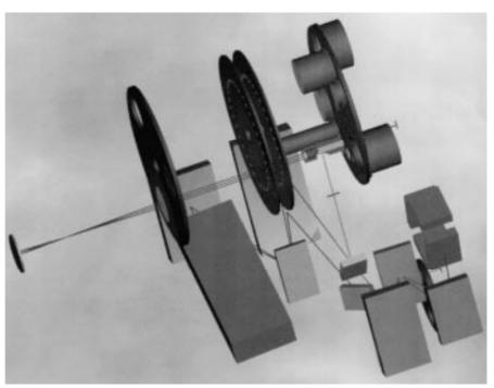
Figure 1: Optical layout of VISIR.
