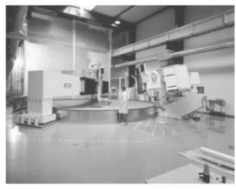
Figure 2: Mirror No. 2 in the grinding stage.
