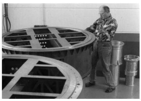
Figure 2: Incoming inspection of the FORS1 and FORS2 top sections; they will house the multiobject spectroscopy units. At right are the tubes of the collimators for FORS1 needed to change the image scale.
