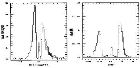
Figure 6: Distribution of statistical errors computed by MINUIT. Left: errors on column density; right: errors on Doppler parameter. Solid line is from the MINOS procedure, dashed line from the HESSE procedure. Note that a fraction of errors estimated with HESSE are implausibly small. Data are for 1000 saturated lines of b = 20 and  $\log N = 15$ .
