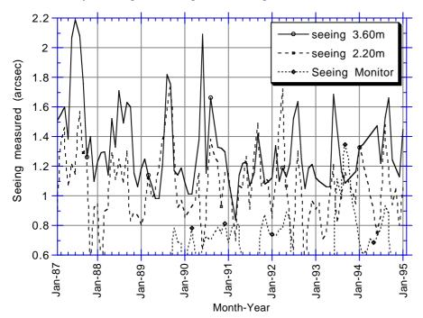
Figure 1: Seeing recorded at La Silla 3.6-m, 2.2-m and seeing monitor telescopes from January 1987 to December 1994.
