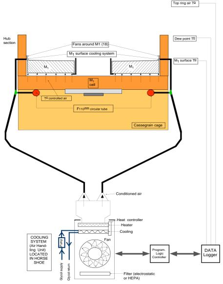
Figure 4: M1 cooling system presently implemented (section).
