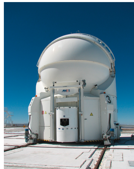
Figure 3. An Auxiliary Telescope with lifted ROS module ready to be moved to a different baseline position.
