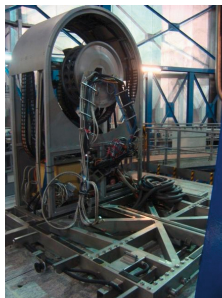
Figure 2. ISAAC, the silver round box in the upper part of the left image, is being taken out from its place at UT1. The right photo shows the co-rotator unit.
