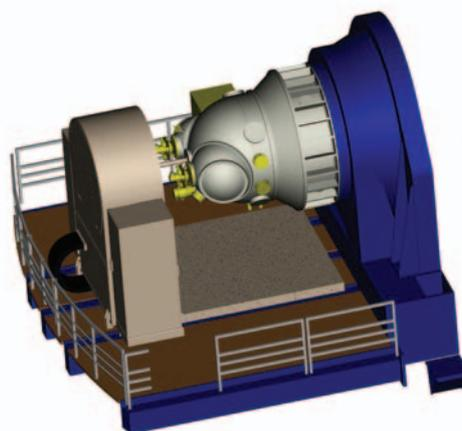
**Figure 2:** HAWK-I installed at a Nasmyth focus. The large port on this side of the vacuum vessel allows easy access to the detector mosaic and the filter wheels without dismantling the instrument.
