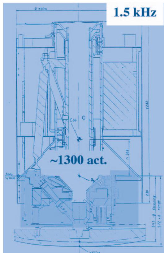
**Figure 5:** Schematic drawing of the M2 unit. The new adaptive secondary system would be put in lieu of the present chopping system (red) and mirror (green). The current focusing (1 d.o.f.) and centering (2 d.o.f.) systems would be kept.
