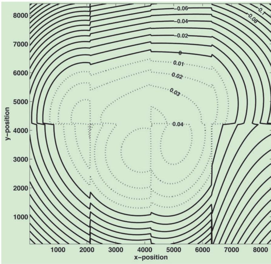
**Figure 2:** Best-fit second-order calibration map after removal of the mean offsets that arose from different flatfield scale factors. The map for the R-band is on the left, the right panel shows the correction map for the V filter. Contours are separated by 0.01 mag. Near the centre of the camera, stars are measured fainter than near the edge.
