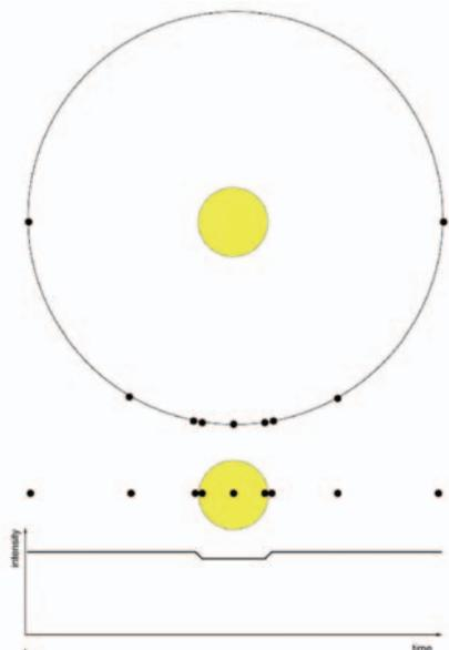
Variations in stellar brightness and velocity, caused by an orbiting exoplanet that transits the disk of its central star. Consecutive positions of the planet in its (circular) orbit are marked by black dots, with the motion from left to right.
