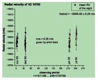
Figure 6: Radial velocity of HD10700 (Tau Ceti) taken for determin ing the long-term accuracy of FEROS. After monitoring the radial velocity of this constant star for almost one year (245 days), we obtain an rms of 8.28 m/s of constancy.
