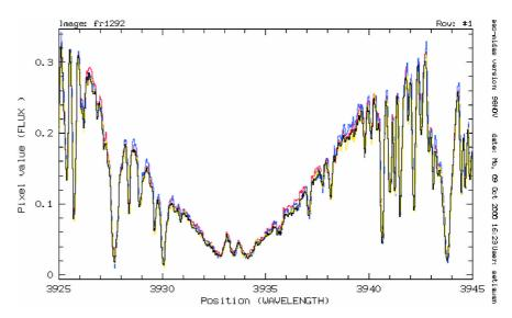
Figure 1: Ca II K line observations of one of the target stars. Observations taken in different nights are overlapped. In case of rotational modulation induced by surface inhomogeneities, the chromospheric core of this line will show detectable variations.
