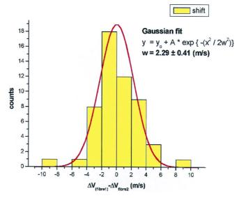
Figure 5: Determining the FEROS calibration stability by checking the shifts between fibre 1 and fibre 2. 50 Th-Aexposures have been tak en for this purpose; the results indicate and RMS of 2.3 m/sec.
