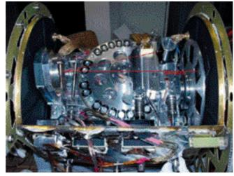
through the (encapsulated) polariser unit to the filter wheel, cold stop and lens wheel, then to the detector unit which is mounted to the back of the bench. The distance aperture/slit wheel to collimator is  $\approx$  350 mm. Three drive shafts are clearly visible, from left to right: filter-wheel, polariser movement and polariser insertion.
