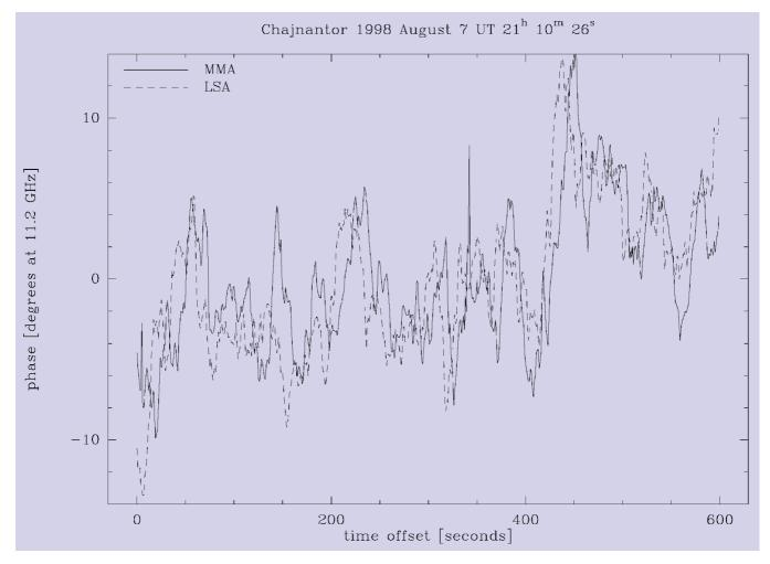
Figure 12: Example of the 11.2-GHz interferometers data showing the expected time delay as the atmospheric turbulence patterns cross over the interferometer line of sight. From these data a height of about 500 m for the turbulence layer can be inferred.
