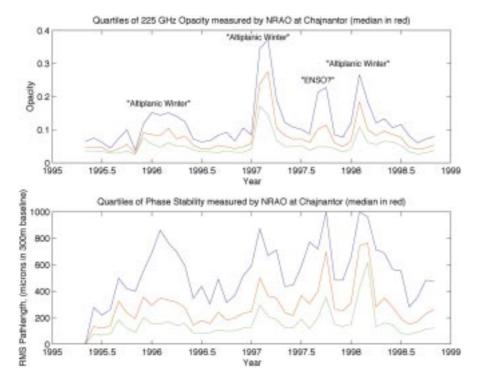
phase errors between the array elements which degrade the sensitivity and resolution of the images. To minimise such atmospheric degradation, then, the ideal site should be a dry plateau at high altitude.
