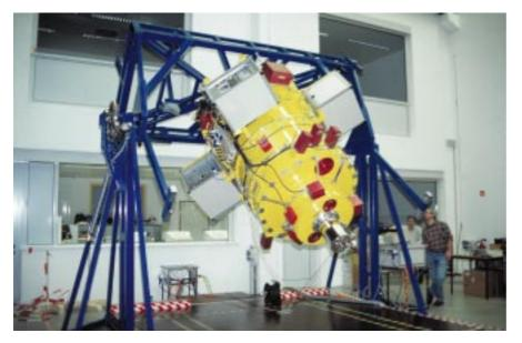
Figure 2: FORS1 on the telescope simulator during flexure tests in the integration hall of DLR at Oberpfaffenhofen near Munich.
