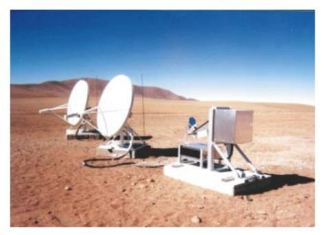
Figure 4: One of the 183-GHz water vapour monitors to the right of the antennas of the 11.2 - GHz interferometers.
