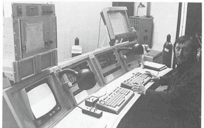
Fig. 1: The observers desk at the 1.52 m telescope with the IDS control equipment.
