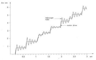
Fig. 3. — Simulation curve showing how the servo system behaves during tracking if the bearing friction is too high.
