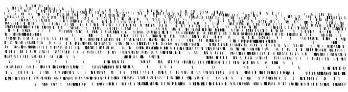
A part of the mask for the CORAVEL instrument, here shown in negative. Each line corresponds to a line in the spectrum of a late-type (cold) star. More than 3,000 lines were drawn by a computer programme operating the ESO S-3000 measuring machine in Geneva in a play-back mode. The mask is enlarged several times in this figure.
