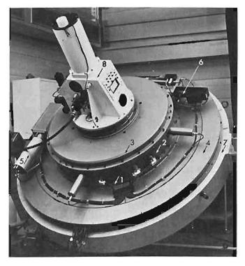
Fig. 1: CASSEGRAIN INSTRUMENT ADAPTEA ON TEST BENCH. — (1) rotator, (2) adapter housing, (3) reduction plate, (4) cable guide. (5) TV camera for contreliald observation, (6) ISIT camera for guiding, (7) test bench, (8) spectrograph.
