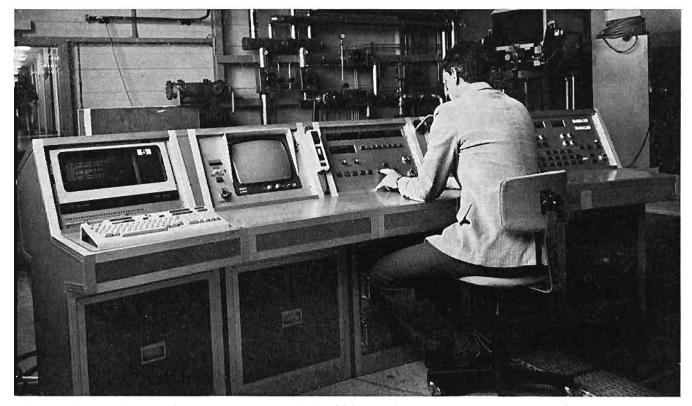
Main desk of the ESO 3.6 m (elescope control system in the ESO assembly hall before departure to La Silla.
