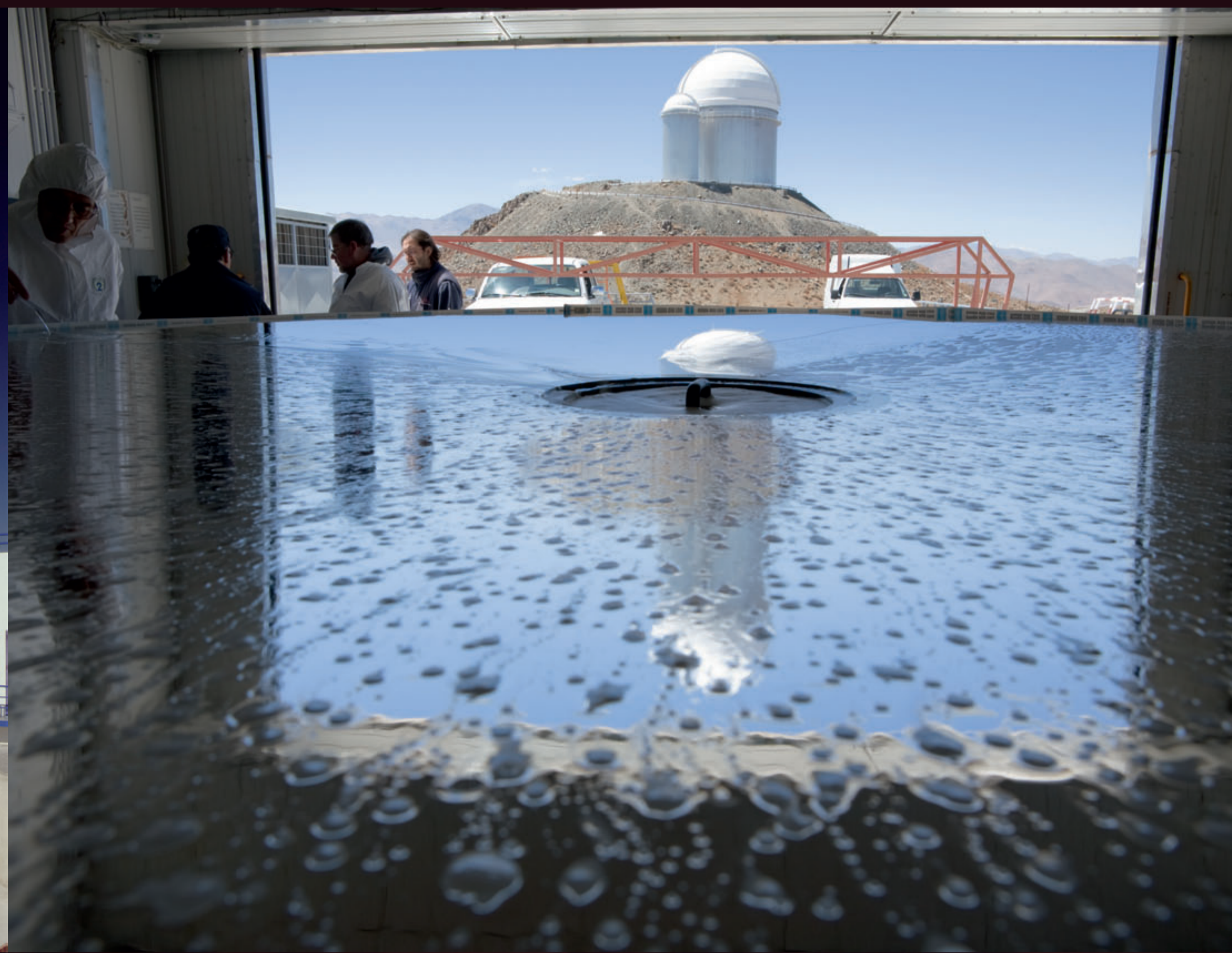
The main mirror of the NTT is removed from the telescope about twice a year for cleaning. Credit: ESO/H.H. Heyer
