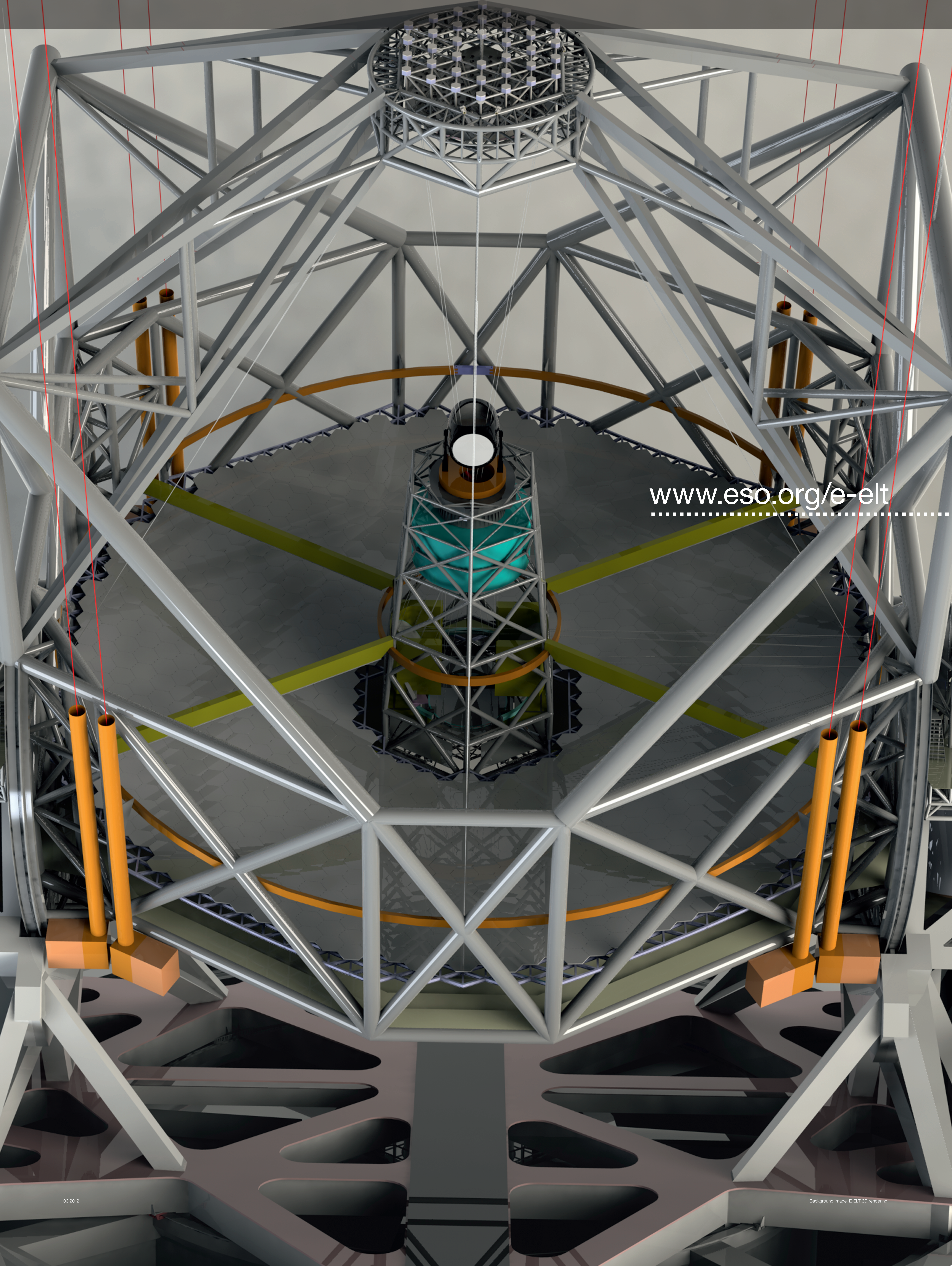
Schematic view of the E-ELT, showing the path light takes through its five-mirror design.
