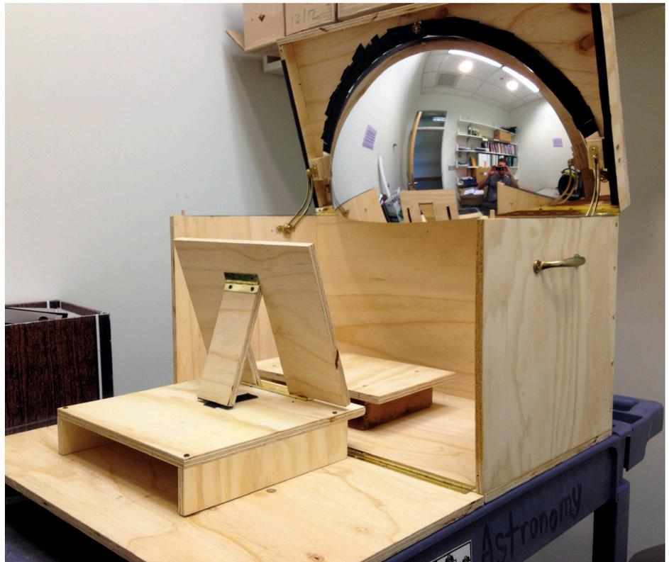
Figure 2. The optics box in the mobile planetarium. The do-it-yourself guide to building the above optics box is available on our website<sup>4</sup>.
