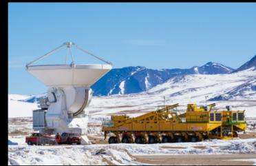
One of the Atacama Large Millimeter/submillimeter Array (ALMA) antennas stands next to Lore, the ALMA transporter. Lore moves antennas between Chajnantor and the lower altitude Operations Support Facility for maintenance.
