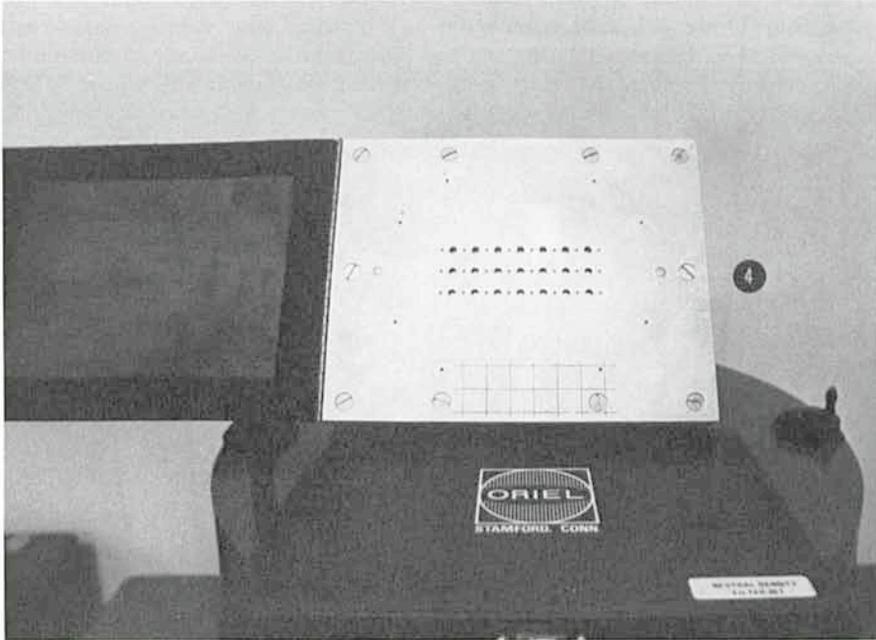
Fig. 4: The exit hole pattern of the tube stack. The grid on the lower part of the plate is for guiding the PM head during photoelectric calibrations.
