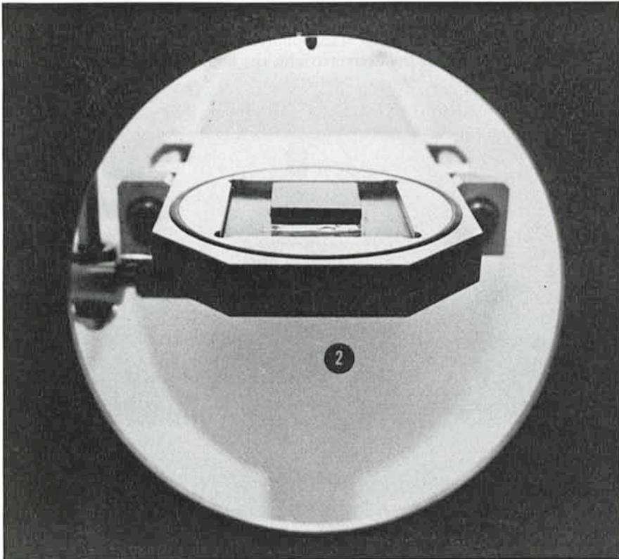
Fig. 2: The filter/diaphragm frame in loading position.
