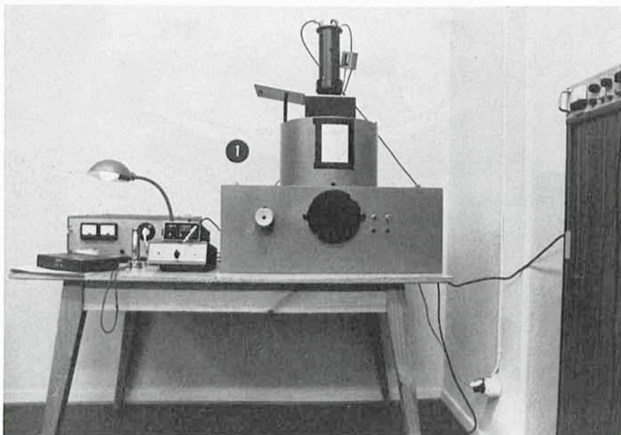
Fig. 1: The ESO spot sensitometer with photoelectric calibrator on La Silla.
