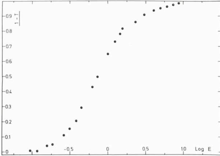
Fig. 6: The characteristic curve of II a-O emulsion 2 AO R1G1/5151 from coude camera III plate "T 5" developed 15 m in D-76. Details of the exposure are given in the text.
