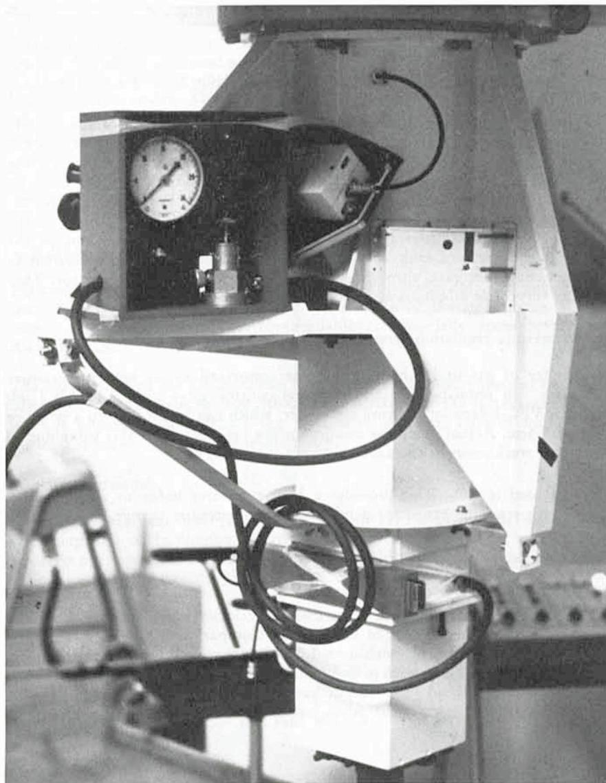
Fig. 2: The Fabry-Perot emission line scanner.
