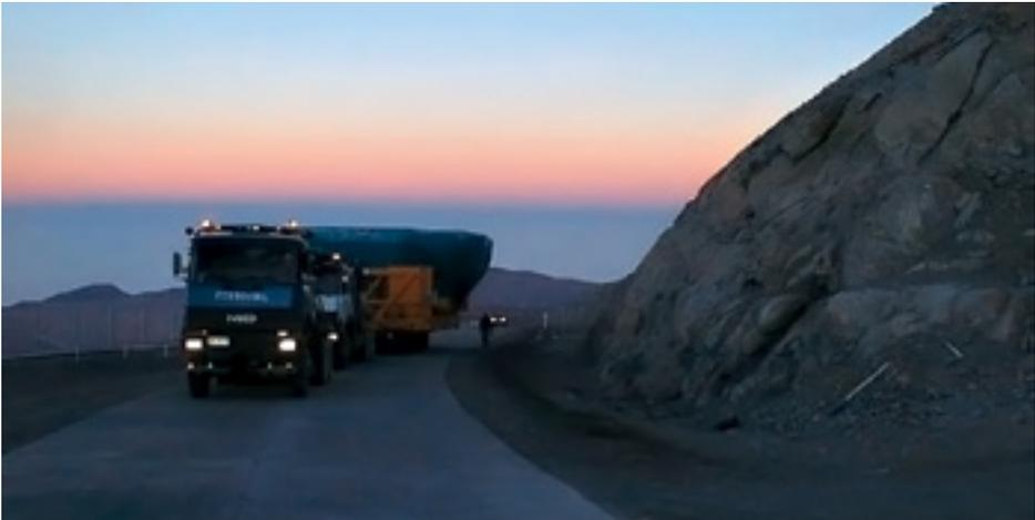
*The primary mirror with its cell is brought up to UT1 after the successful aluminisation on 21 May. In his logbook, Peter Gray noted: “Started operation at 5 am this morning. Moved outside on air cushions 20 min, loaded onto trailer and rigged 40 min. Departed MMB [Mirror Maintenance Building] at 6 am as planned. 1.5 hr transport, arrived UT1 at 7:30 am.” (Photo: Peter Gray)*
