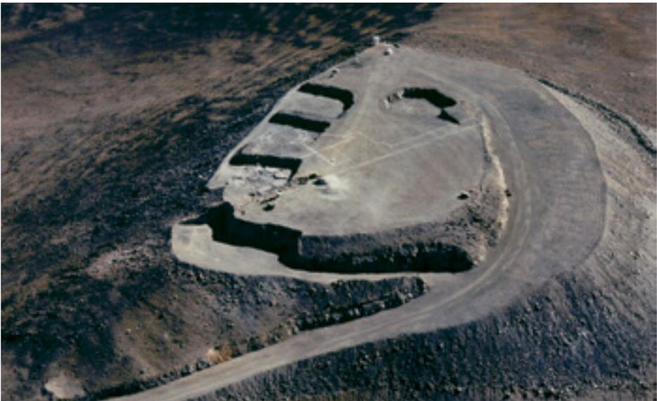
*The layout of the four VLT Unit Telescopes as well as the underground tunnels are clearly visible in this aerial photo, obtained in 1994. (Photo: Herbert Zodet)*
