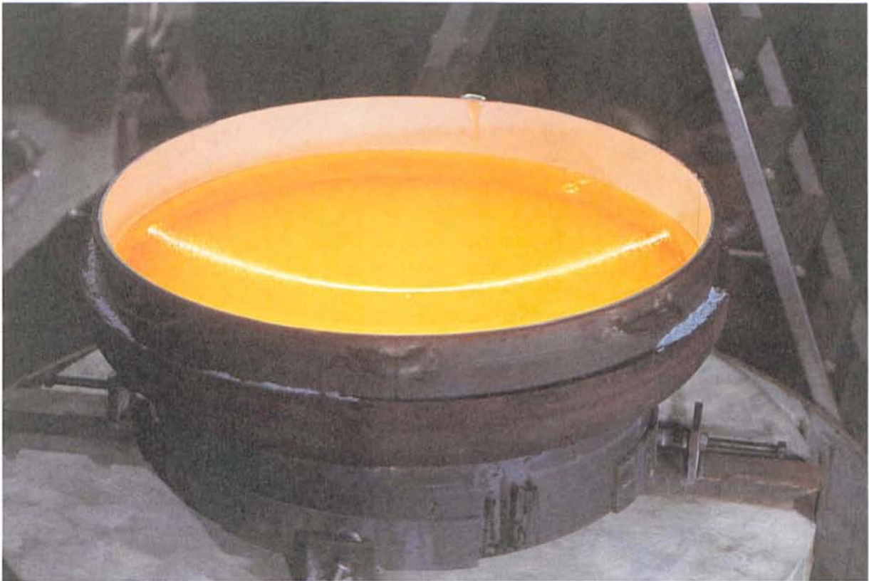
Figure 5.2: Spin cast thin meniscus. The glass in the rotating mould is still fluid.
