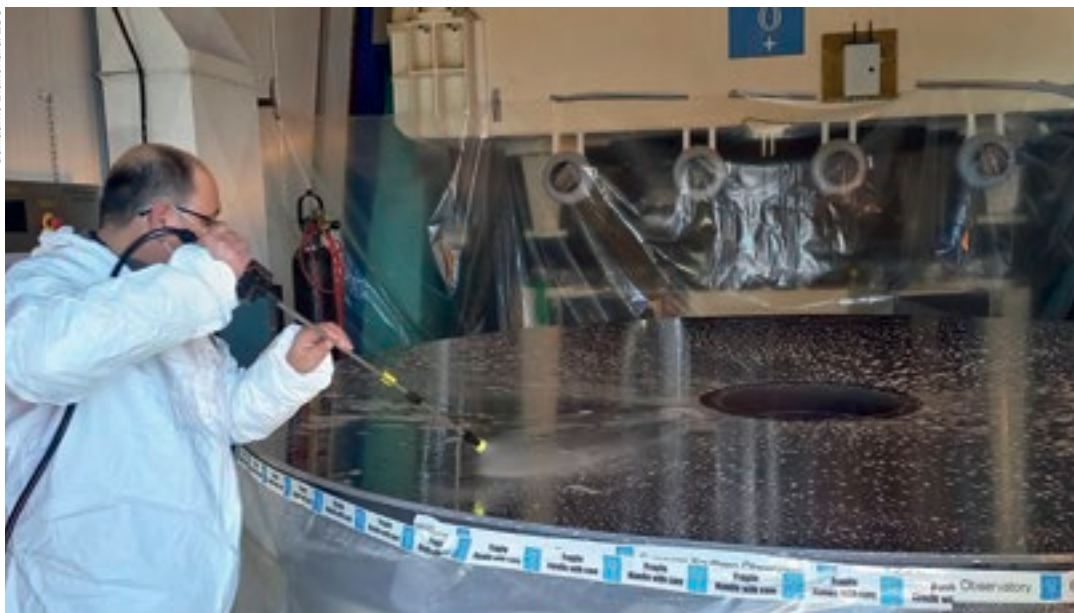
Testing high-pressure washing of the NTT mirror.
