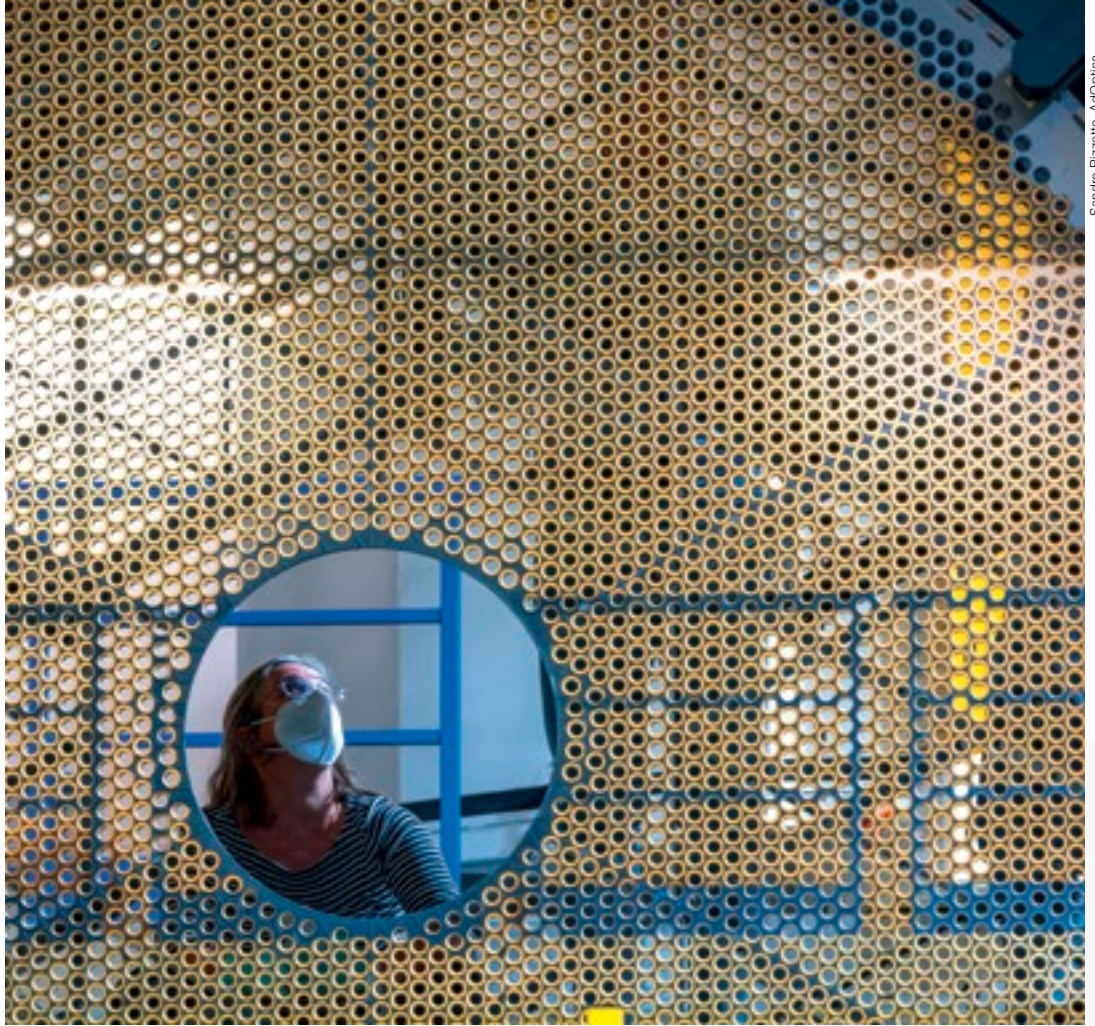
The ELT M4 mirror reference body.
