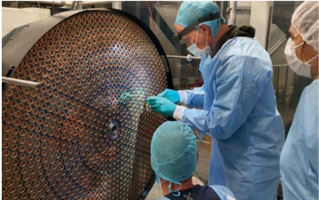
Working on the exchange of the deformable secondary mirror of the VLT's Unit Telescope 4.
