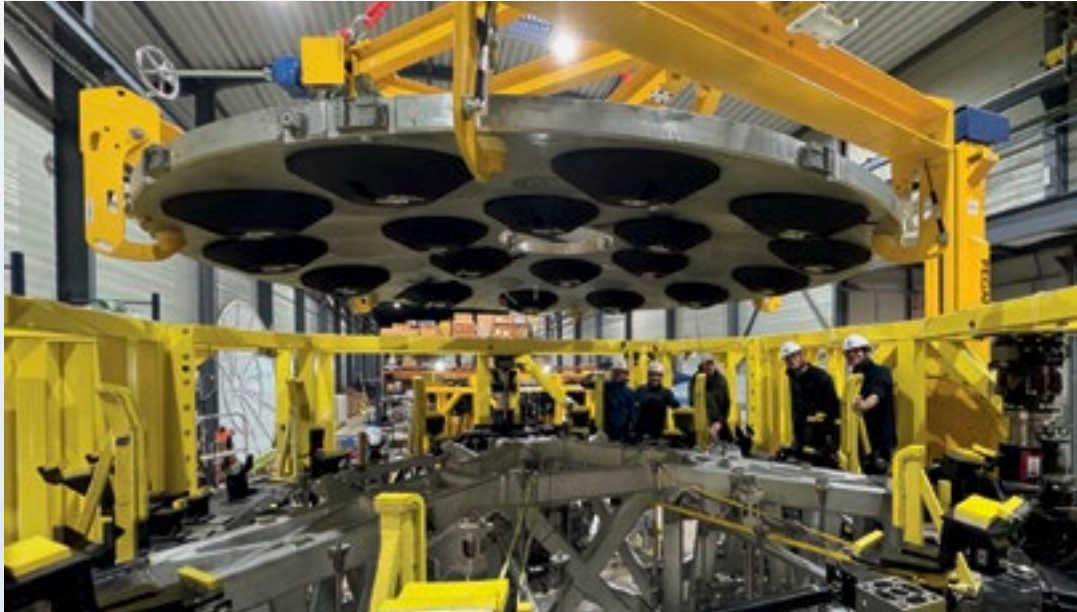
Integration of the dummy ELT M2 mirror on the M2 support cell.
