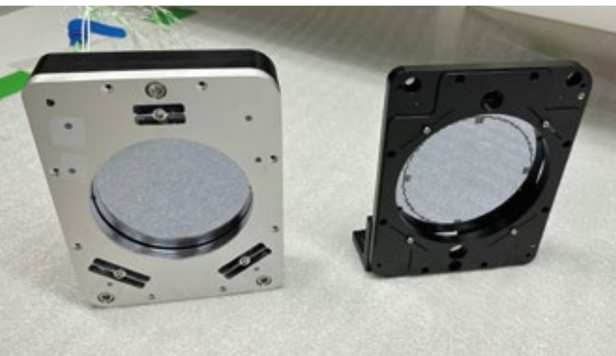
Actuator plate prototypes for the MAVIS deformable mirror.
