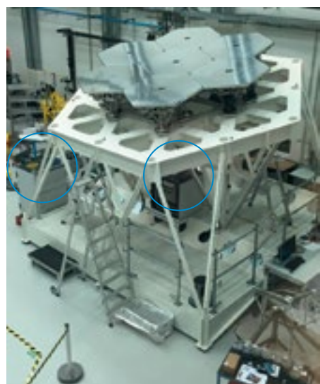
ELT M1 Test Stand with electronics cabinets, the M1 Segment Concentrator Cabinet (circled, on the right) and the Sector Distribution Cabinet (circled, on the left).
