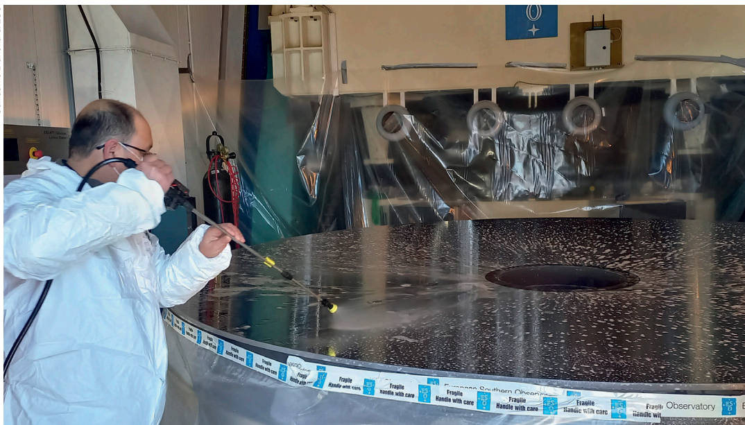
Testing high-pressure washing of the NTT mirror.
