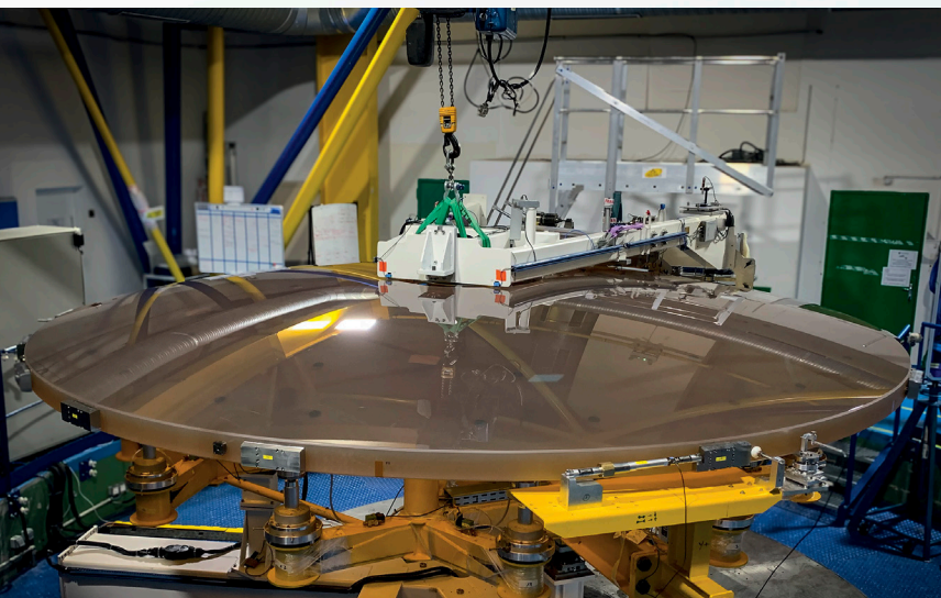
Testing the polished ELT M2 mirror.
