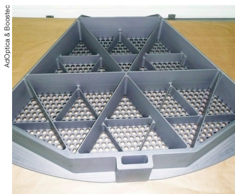
The test version of the silicon carbide M4 support structure.
