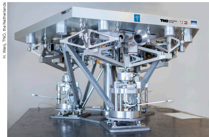
Engineering model of the M1 segment support system (with an aluminium dummy segment) as designed and developed by VDL/TNO.
