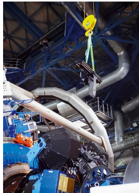
Installation of the ESPRESSO M4 mirror unit on VLT Unit Telescope 3.
