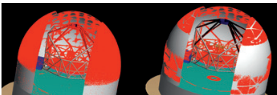
This shows (in red) the surfaces of the dome and the structure that can be seen from the focus through, as examples, the mirrors M1 and M4.
