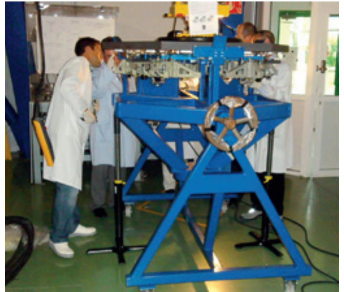
Segment integrated with its support before final polishing.
