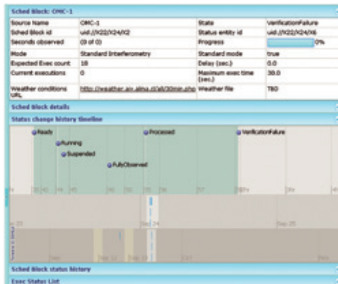
The ALMA project tracker, showing the execution of an observing unit (Scheduling Block) from the time it is first ready to run, through its execution, the processing of its acquired data, up to verification of its quality by ALMA staff.
