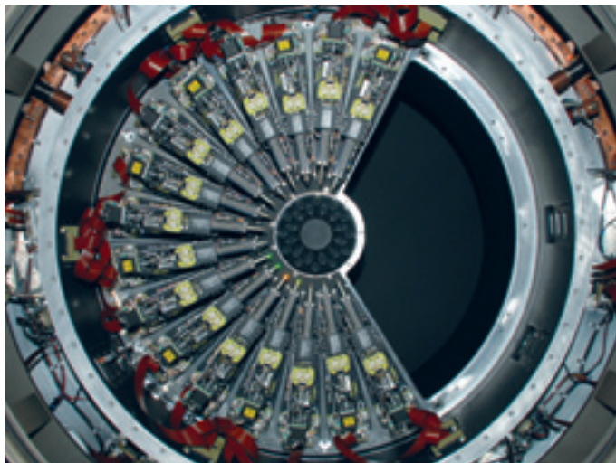
The picture shows 16 cryogenic pickoff arms in the KMOS focal plane. Eventually, 24 will be installed.
