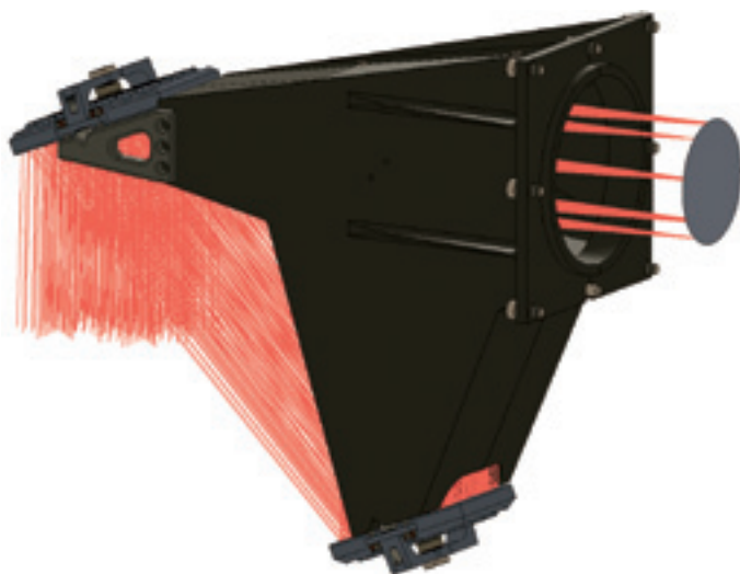
The AO system GRAAL, used for HAWK-I. The red lines show the laser-tracker used to measure the position of key points of the instrument.
