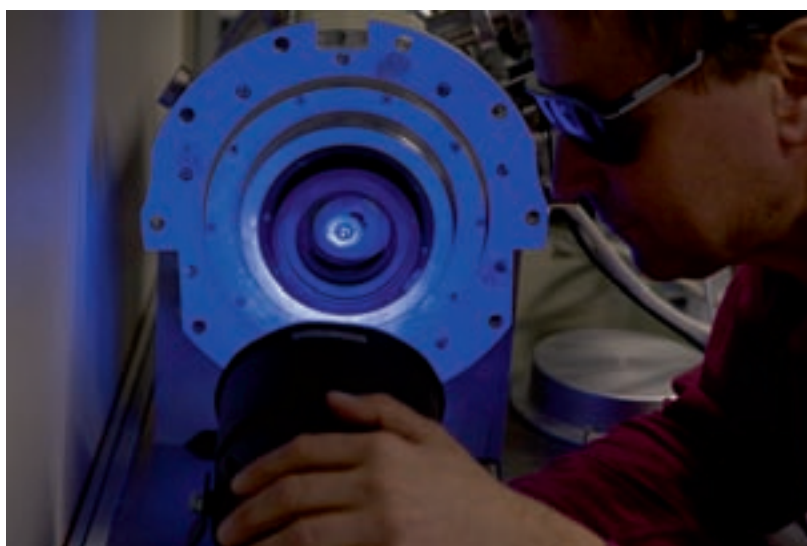
Gas treatment with UV light to improve the quantum efficiency of the FORS1 CCD.
