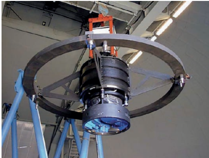
The new 3.6 F/35 unit being mounted on the Serrurier.
