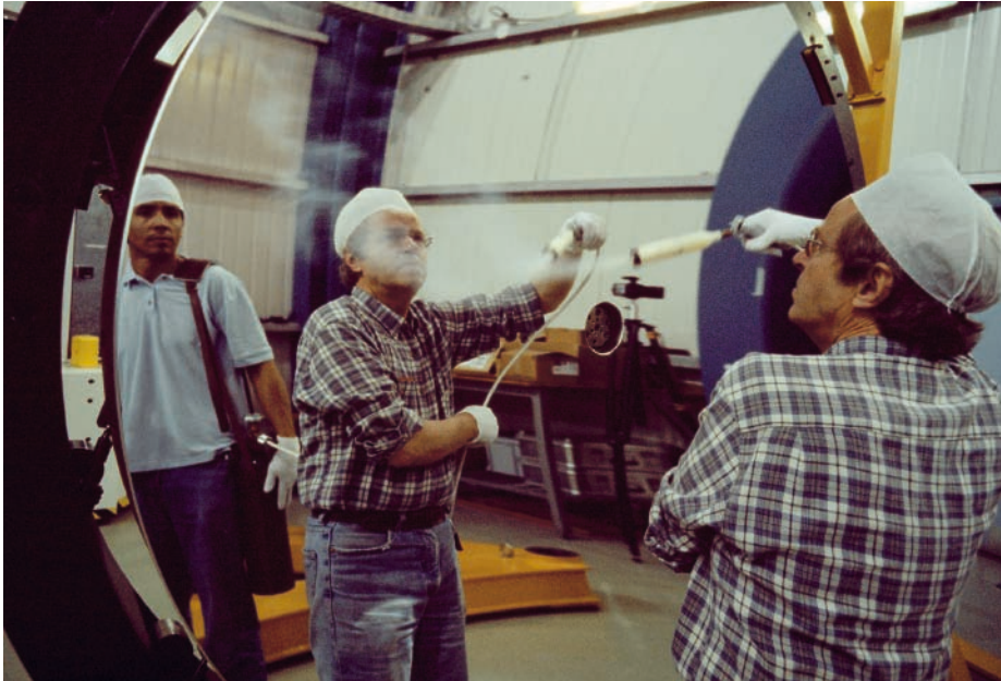
CO 2 cleaning of the AT2 primary mirror.
