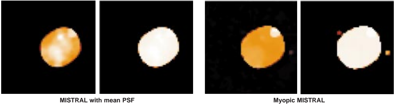
Figure 6: MISTRAL classical deconvolution with mean PSF considered as the true PSF and myopic deconvolution. In each case we show the corresponding log-scale map. The deconvolution is performed on the 0.8 arcsec field of view but only a 0.4 arcsec sub-field is displayed. The distance to the true object is respectively 23,000 and 6800 photons/pixel (see Section 4).
