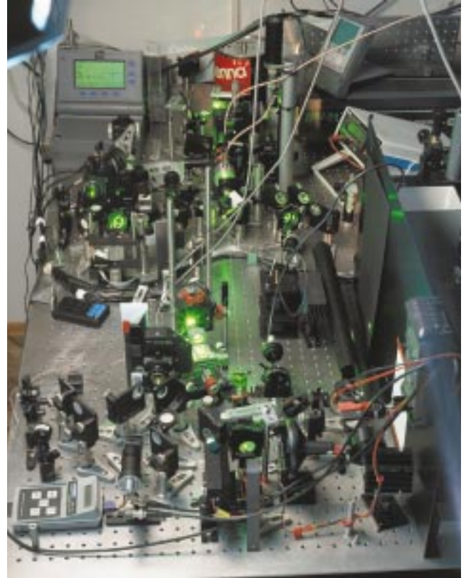
Figure 11: View of the laboratory setup where the fibre experiments have been carried out. The setup allows the measurement of the spectrum, power and propagation properties of the laser beam. The injection, fibre output and SBS return beams can also be characterised.
