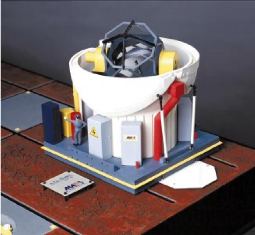
Figure 3: A model of an Auxiliary Telescope during Observations. The 1.8-m telescope (with an Alt-Az mount like the Unit Telescopes) is rigidly anchored to the ground by means of a special interface. The light is directed via the Coudé Optical Train to the bottom of the Telescope. From the Coudé Relay Optics it is sent on to the underground Delay Line Tunnel
