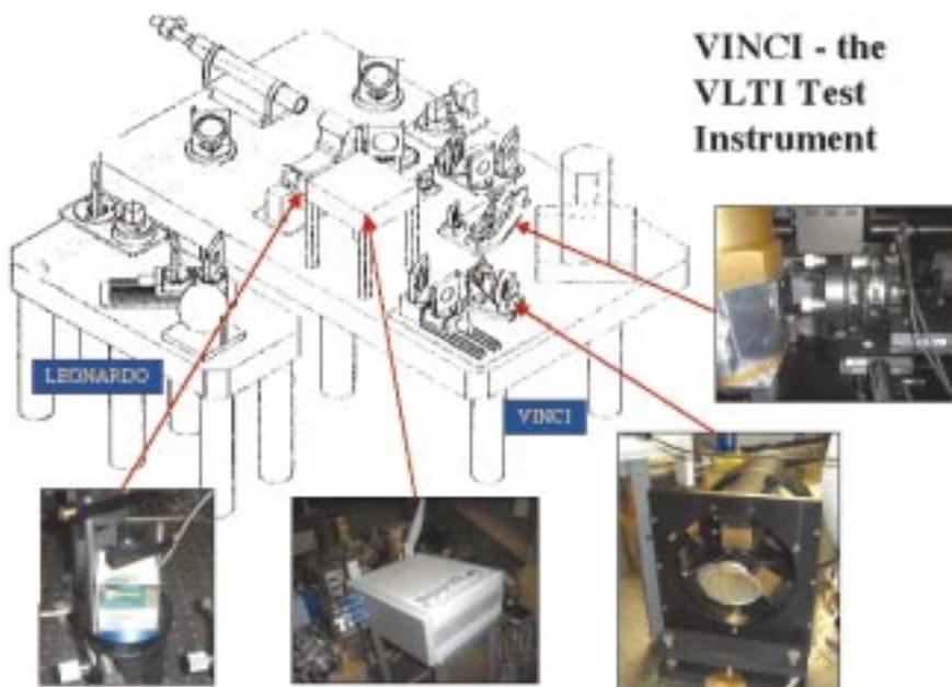
Figure 5: The concept of the VLTI commissioning instrument VINCI. The beam combining unit, VINCI, and the reference source unit, LEONARDO, are placed on individual tables. Their respective positions in the VLTI Laboratory are shown in Figure 4. The main elements on the VINCI table are the fibre beam combiner and the dewar of the infrared detector. The inserted photographs show details of the FLUOR instrument at the IOTA interferometer. VINCI is a conceptual copy of FLUOR.
