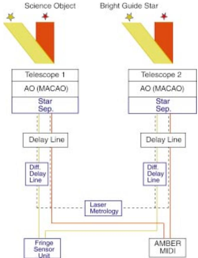
Figure 7: Functional block diagram of the VLTI and the PRIMA components. The VLTI has the following subsystems: Telescope 1 and 2 – two UTs or two ATs, AO – Adaptive Optics, Delay Lines, AMBER/MIDI – Science Instruments. The PRIMA subsystems are: Star Separator, Differential Delay Line, Laser Metrology, Fringe Sensor Unit.
