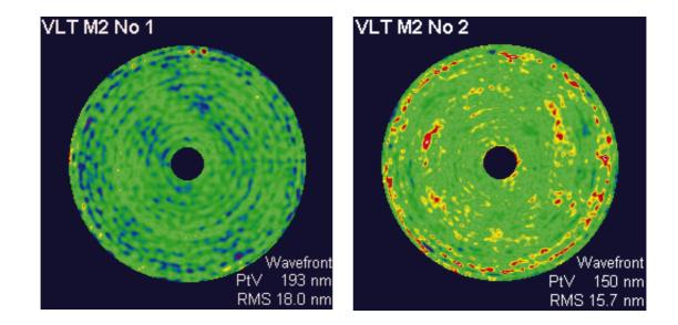
spections were also performed. The surface quality of both mirrors is excellent and within specification.
