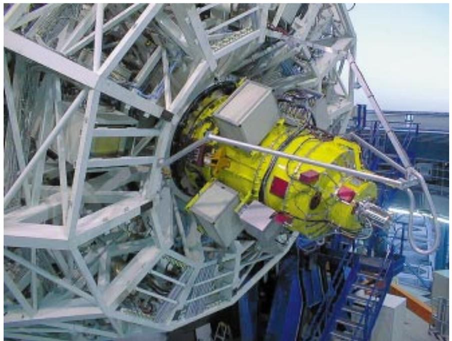
Figure 1: FORS1 installed on UT1. The instrument with the electronics boxes is well visible as well as the tripod on the M1 cell that carries the cable hose. This cable hose (a flexible metal hose) contains all electric power, LAN and cooling water lines for FORS.
