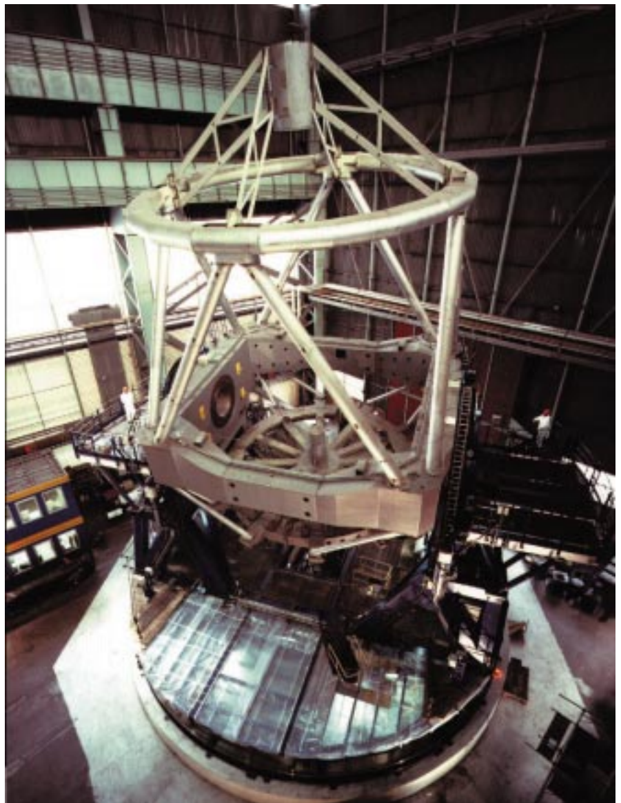
The VLT mechanical structure during the tests at the Ansaldo factory in Milan, Italy.
