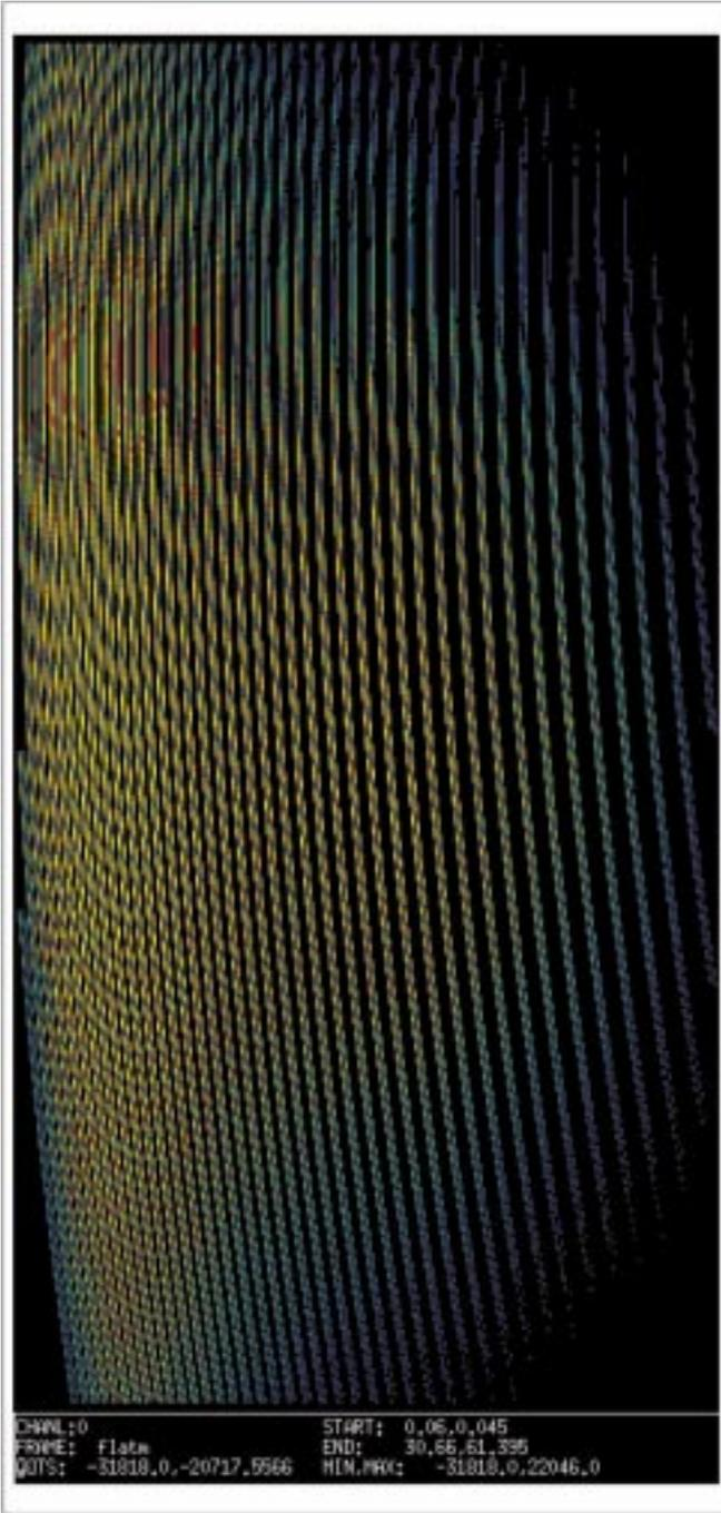
Figure 2: Spectral format of FEROS showing a simulated flatfield exposure. Red is to the left with the extreme order 32 with  $\lambda_c = 9850 \text{ \AA}$ ; blue is to the right with the extreme order 63 with  $\lambda_c = 3600 \text{ \AA}$ . Each spectral order is double due to the illuminated object and sky fibre. The whole echelle spectrum is rotated counter-clockwise by  $2.4^\circ$  to align the slit image with the CCD rows.
