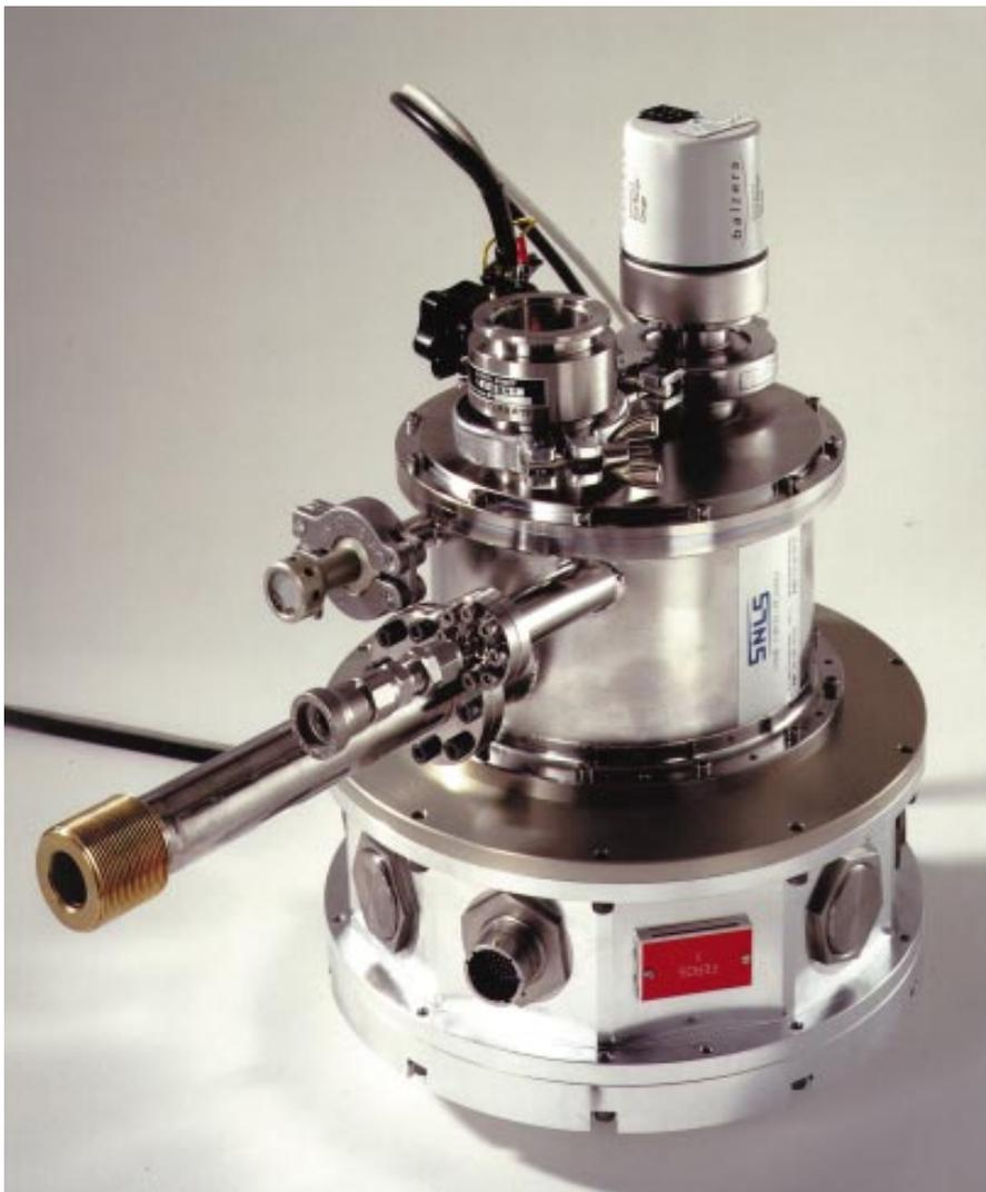
Figure 1 : Continuous-flow cryostat.
