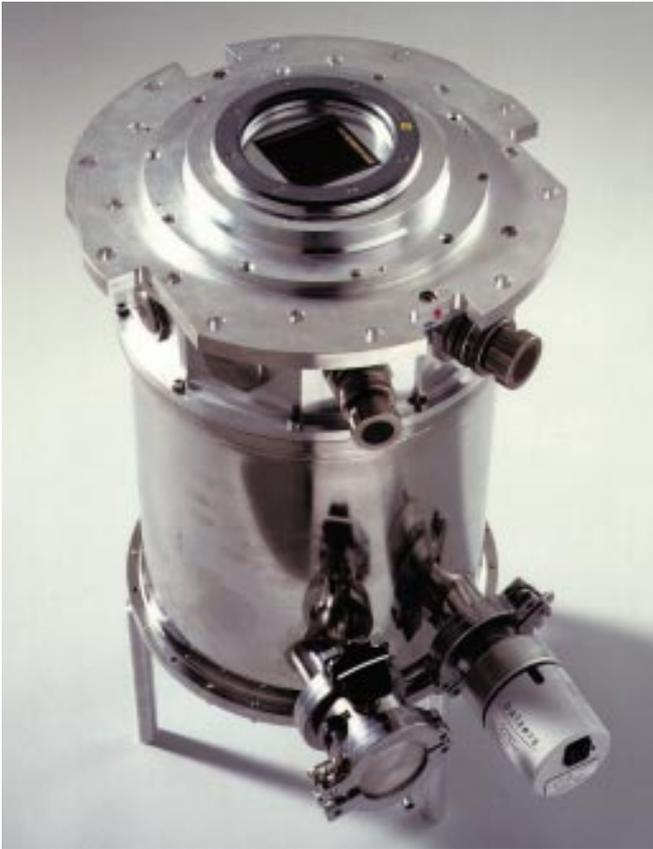
Figure 2 : Bath cryostat, Cassegrain version.
