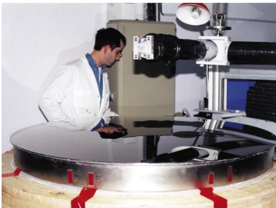
Figure 2: The Beryllium secondary mirror during polishing at REOSC Optique.
