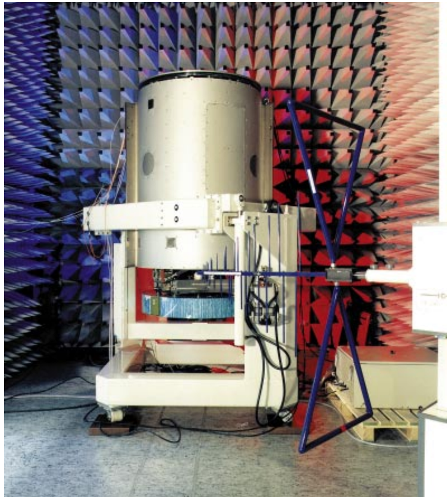
Figure 1: The M2 Unit equipped with the M2 dummy in the anechoic chamber of Dornier. (Photo Dornier).
