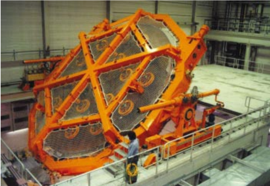
Figure 3: Turning the blank convex side up.
