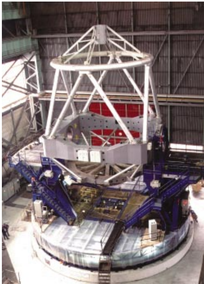
Figure 4 was taken in Milan in October 1996 during the final integration of the telescope structure. The telescope is fully equipped with all subsystems and associated electronics.
