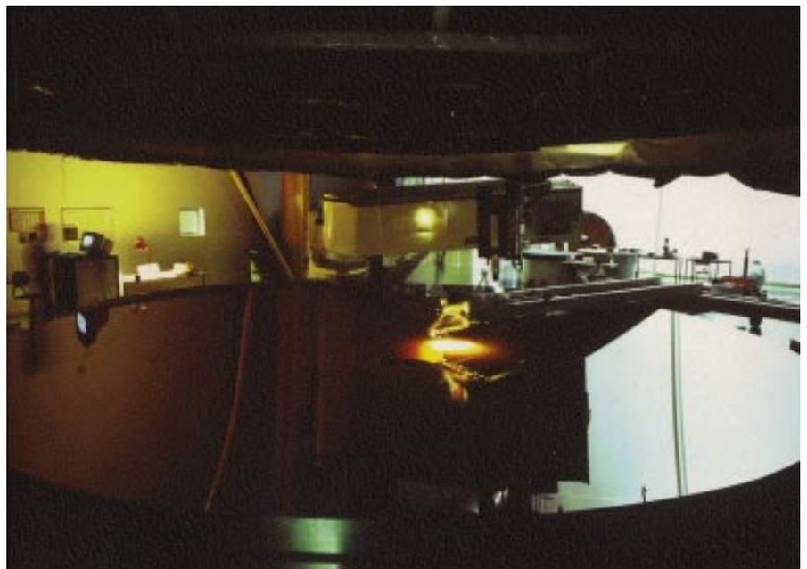
Figure 5: Primary Mirror undergoing acceptance tests at REOSC.
