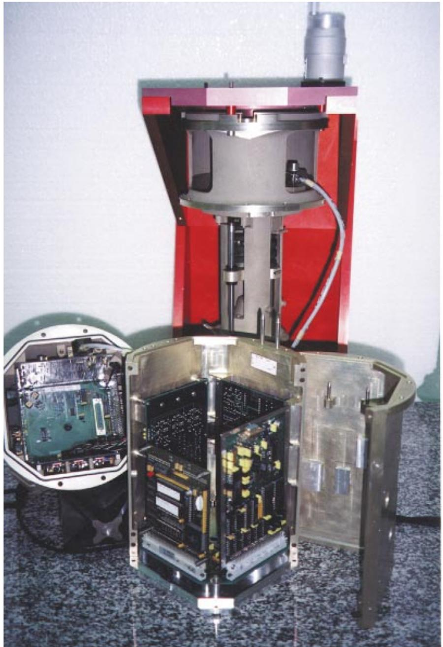
Figure 4: Active axial force actuator.
