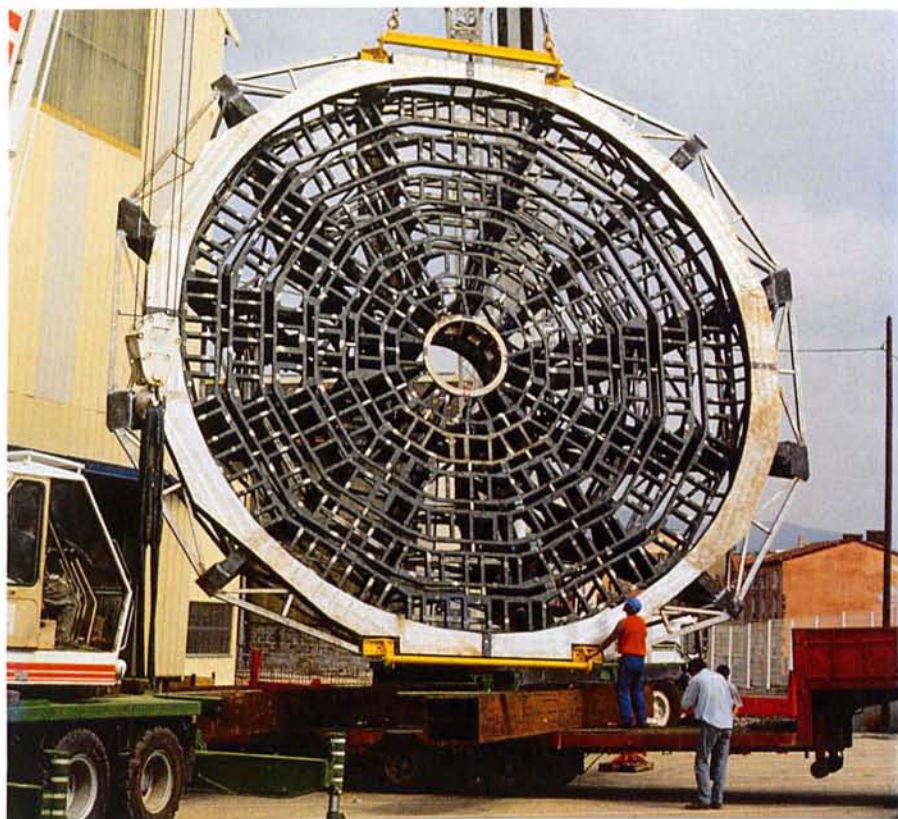
▶ The primary mirror cell of the VLT (Unit 1) is turned at the St-Chamond GIAT factory, prior to undergoing dimensional check and painting (16/07/96).
