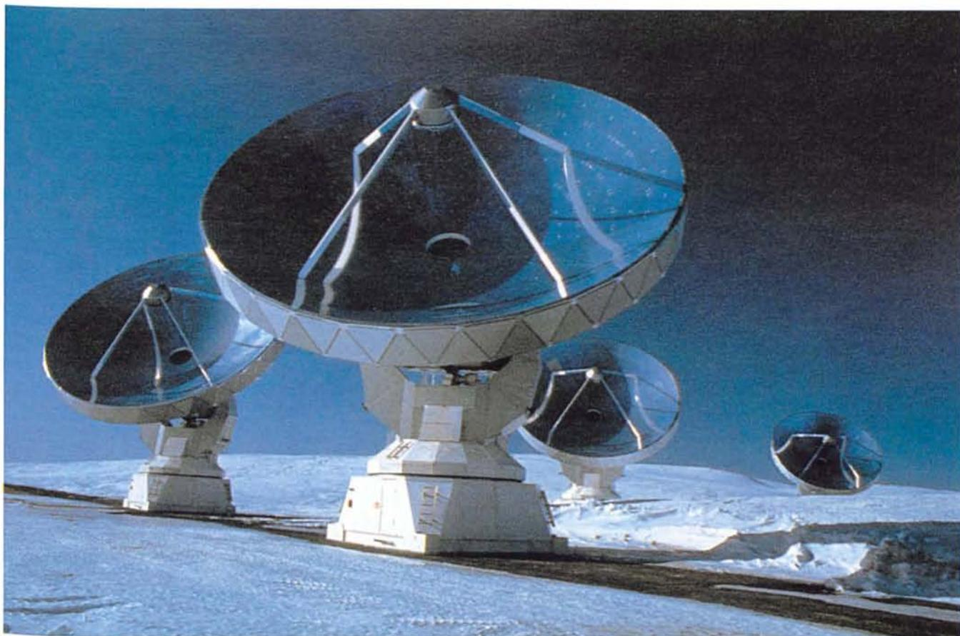
Current state-of-the-art in millimetre arrays: the four 15-m antennas of the IRAM interferometer on Plateau de Bure, France.
