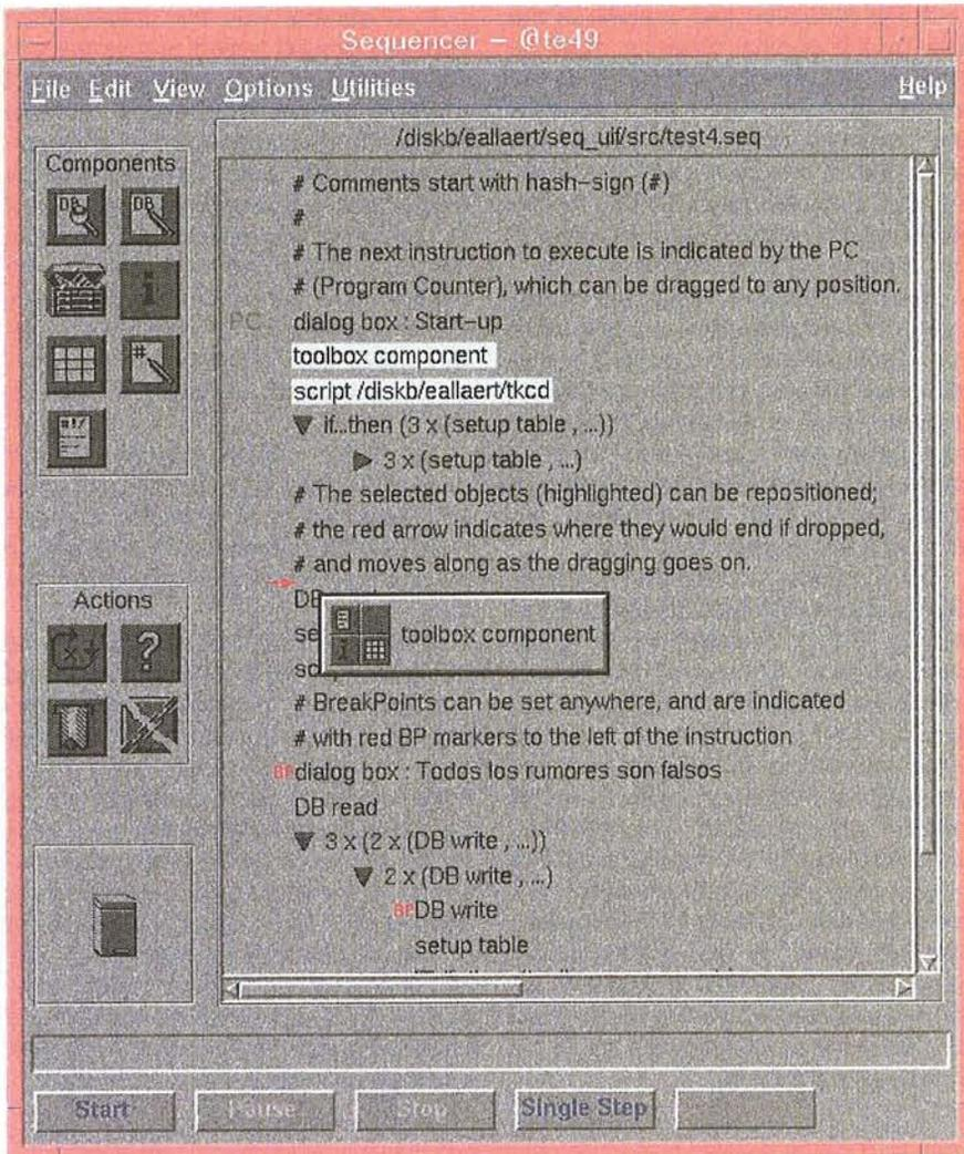
Figure 1: A snapshot of the Sequencer's prototype GUI.
