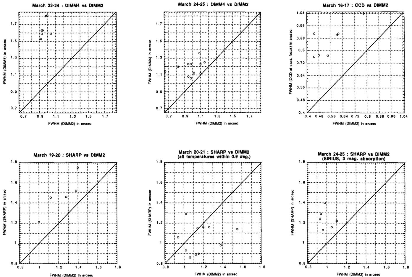
Figure 3: Seeing measurements made on several occasions in March 1995, with M1 cooled to ambient  $T^\circ$  ( $T_a \pm 1^\circ$ ) and floor cooled to  $T_a - 2^\circ$ . Comparison with the seeing monitor DIMM2 gives an estimate of remaining M1 and dome seeing.
