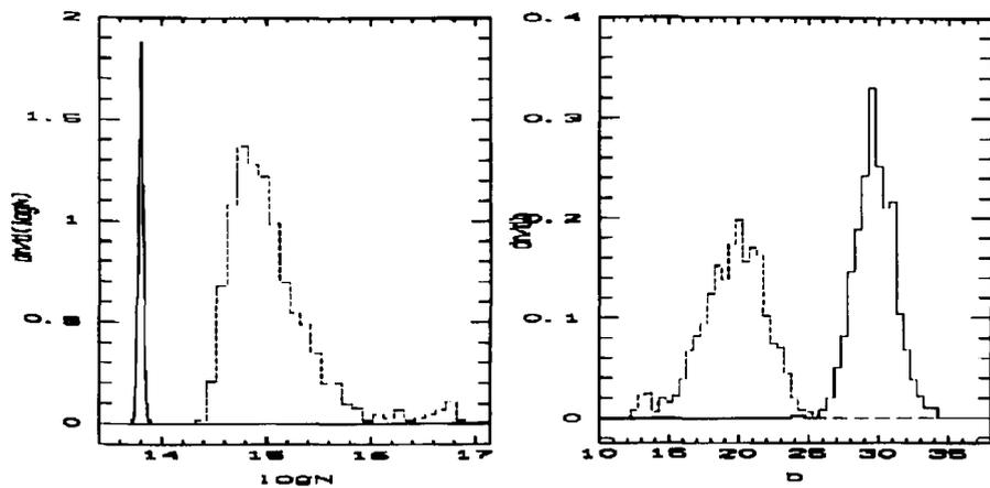
Figure 4: Distribution of Doppler parameter  $b$  (right) and column density  $N$  (left) obtained by the fitting procedure for 1000 lines with  $S/N = 10$ . Solid line is for lines of  $b = 30$  and  $\log N = 13.8$ , and dashed line is for  $b = 20$  and  $\log N = 15$ . Solid line on the left panel has been divided by 10 for illustrative purposes.
