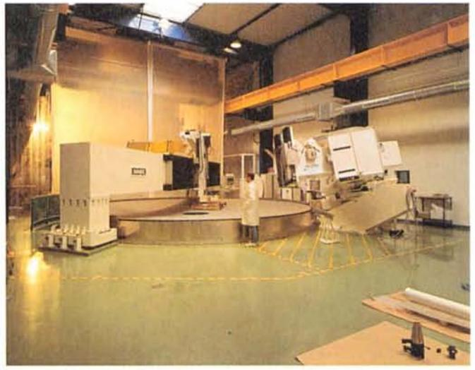
Figure 2: Mirror No. 2 in the grinding stage.
