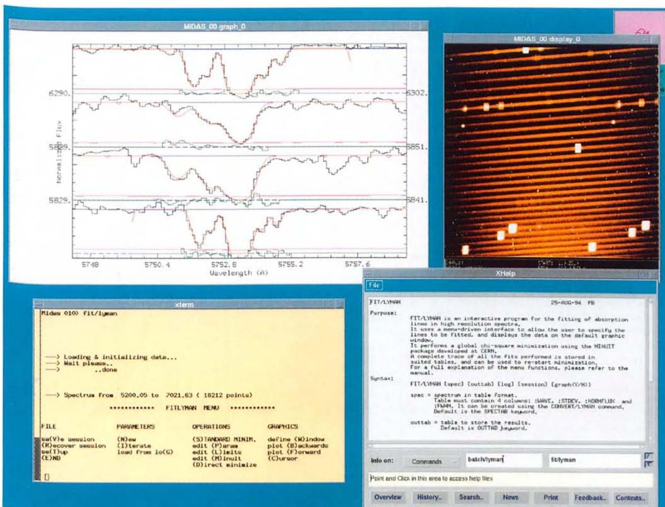
Figure 1: Example of a FITLYMAN session. The Main Menu is shown in the bottom left window. The graphic window over it displays a fit performed on a complex metal system at  $z = 2.768$ . Lines fitted are, from the top, Al1670, CIV1550, CIV1548, SiII1526. The CIV doublet has been fitted with three components, lower ionisation elements with five. Data from Giallongo et al., 1993, and J. Wampler.
