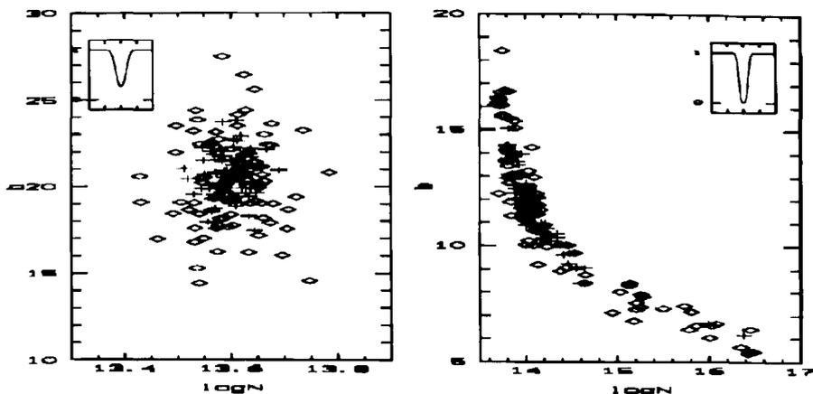
Figure 5: Values of Doppler parameter  $b$  and column density  $N$  obtained by the fitting procedure for 100 lines at different  $S/N$  ratio. Lozenges are for  $S/N = 5$ , crosses for  $S/N = 10$ . Left: an unsaturated line of  $b = 21$  and  $\log N = 13.6$ ; right: a saturated line of  $b = 12$  and  $\log N = 13.8$ . Small boxes show the respective line profile.
