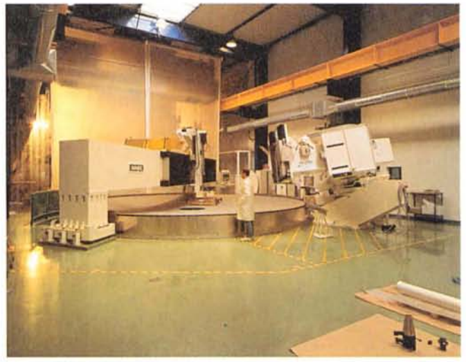
Figure 2: Mirror No. 2 in the grinding stage.
