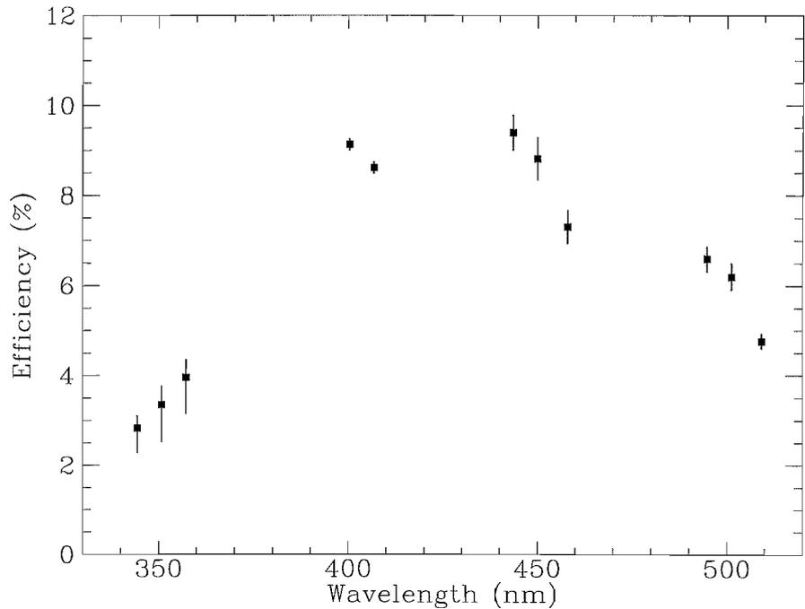
Figure 2: The total efficiency of the NTT, EMMI blue with Grating #11 and CCD#31 as a function of wavelength. The error bars indicate the actually measured values for the two stars observed.
