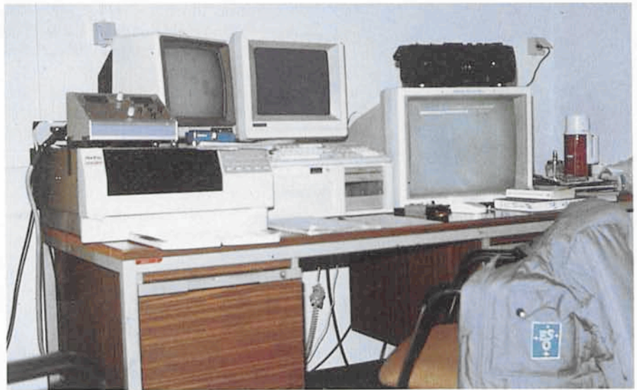
Figure 3: Control room at astronomers office with CCD-, computer- and TV-guiding-monitor, personal computer, and magnetic tape. With this equipment we are completely independent, using only the naked telescope at each observation site.
