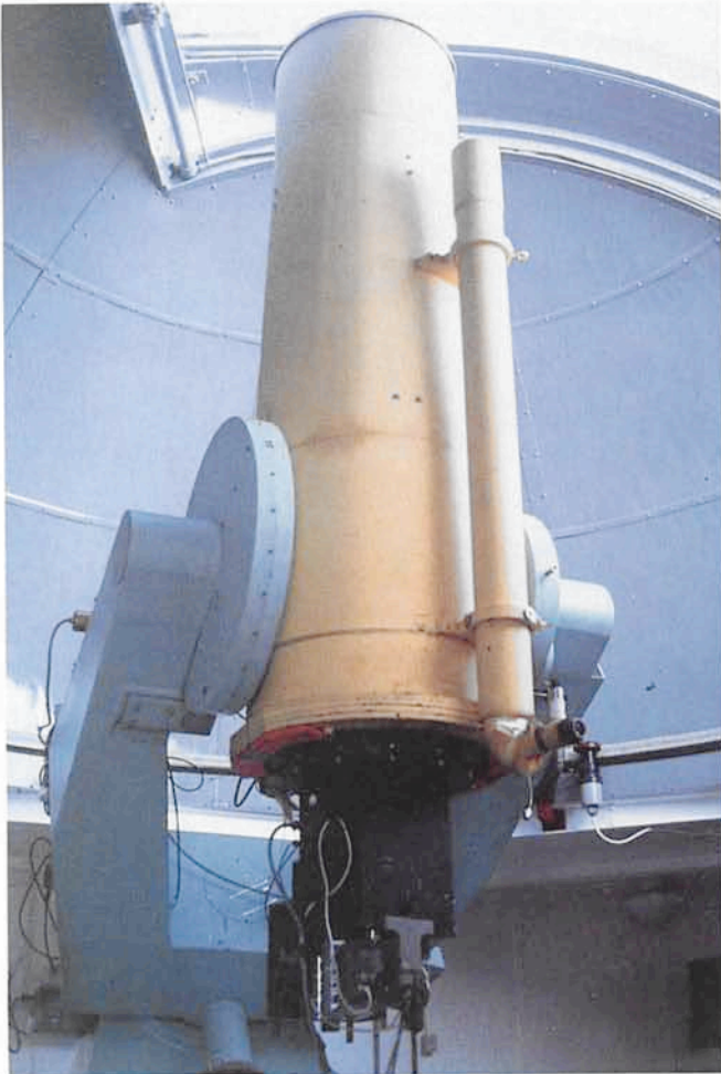
Figure 1: ESO 50-cm telescope with the TV guiding system of FLASH. The total weight of the guiding system is only about 35 kg. It contains the fiber-fed interface, comparison lamps and a conventional SIT low-light-level camera.
