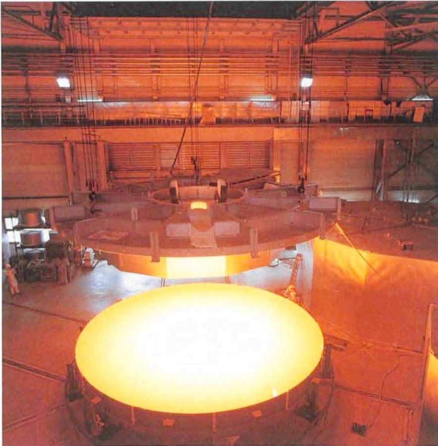
Figure 2: Lifting the overhead heating system.
