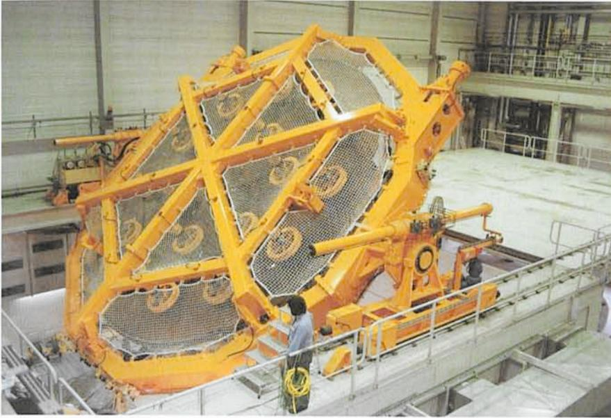
Figure 3: Turning the mirror blank.
