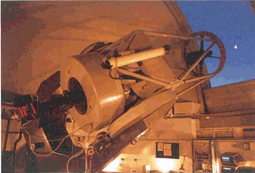
Figure 1: The DLR CCD camera installed at the ESO 1-m telescope.
