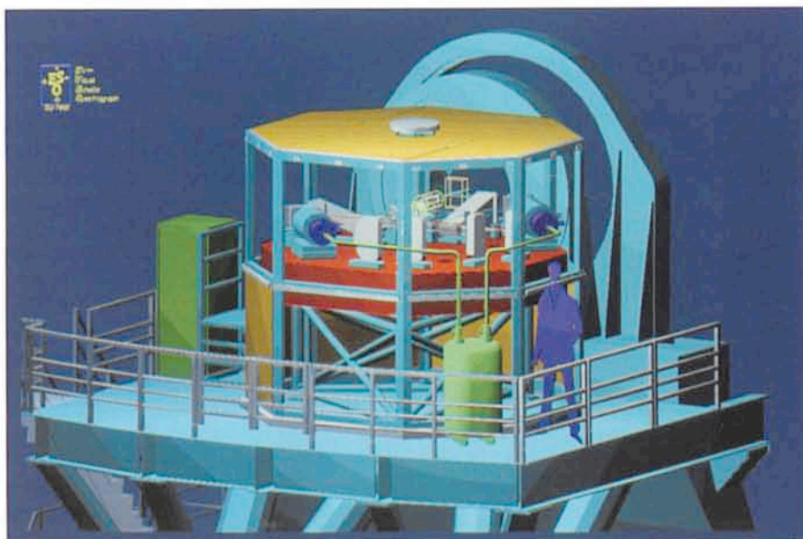
Figure 1: 3-D view of UVES with most of the enclosure panels removed for clarity.
